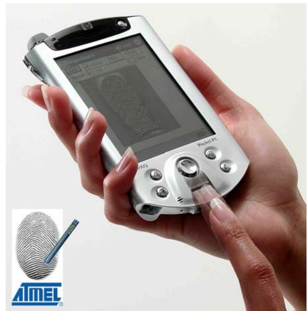
Fig.4 iPAQ Pocket PC h5455 with the FingerChip
